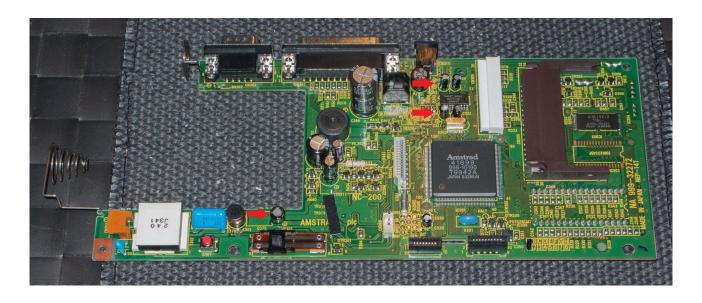
Capacitors marked with an  $\rightarrow$  need to be short otherwise it will not be possible to screw floppy drive and close the case
